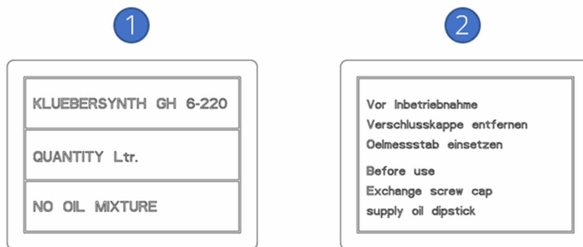
Fig. 1: Labels on intermediate gear box
