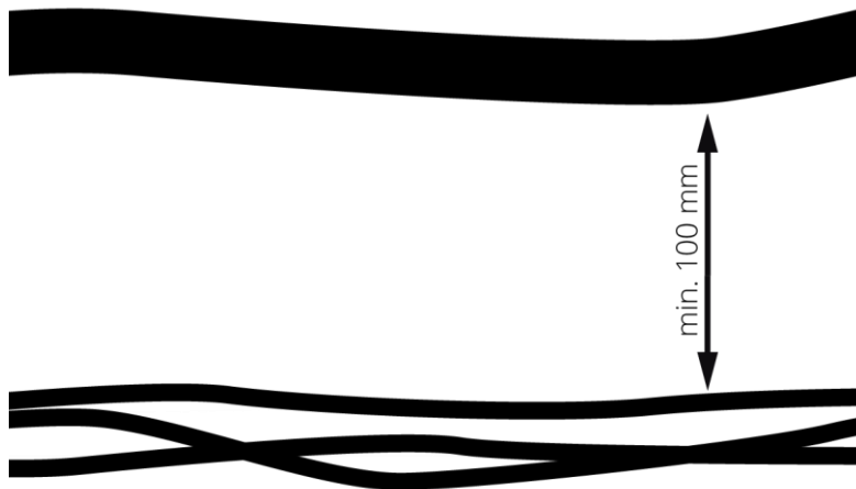
Fig. 7: Minimum distance motor and sensor cables
