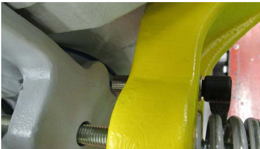
Pic. 2: showing the inductive proximity switch for the Brake Lining Wear control
