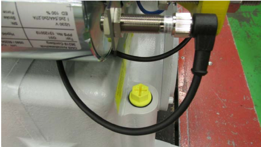
Pic. 1: showing one of the inductive proximity switches for the Brake Function Control
