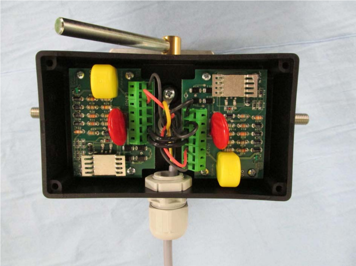
Picture: 022/032 Braking Solenoid, view into the opened junction box shows the electronic control module.
